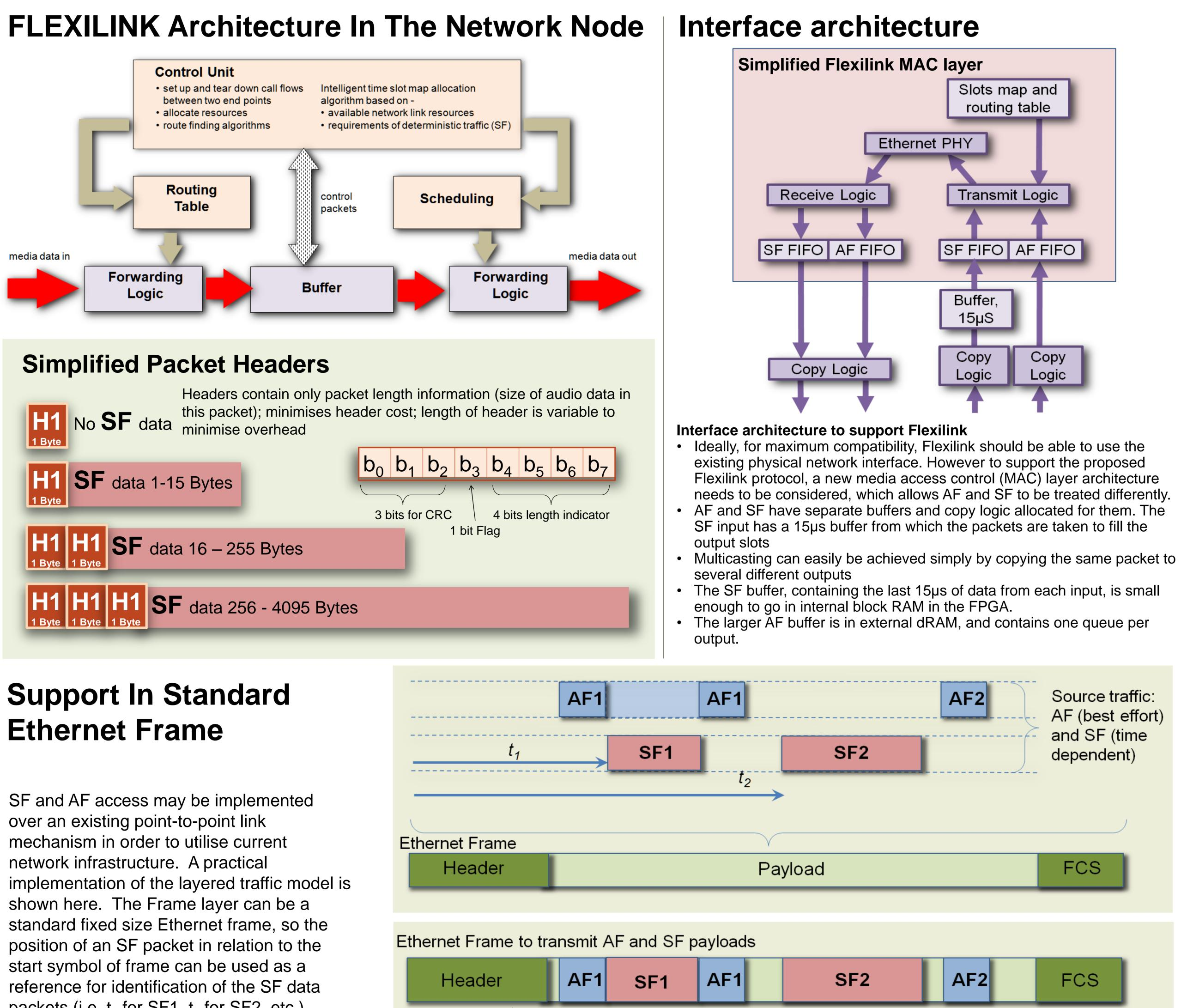
packets (i.e.  $t_1$  for SF1,  $t_2$  for SF2, etc.) Consequently labels for SF identification are not required.
